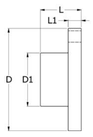
$\begin{array}{lll} D & = 162 \\ D1 & = 85 \\ L & = 60 \\ L1 & = 20 \\ Max \ bore & = 50 \\ Torque \ (N \ m) = 750 \end{array}$
